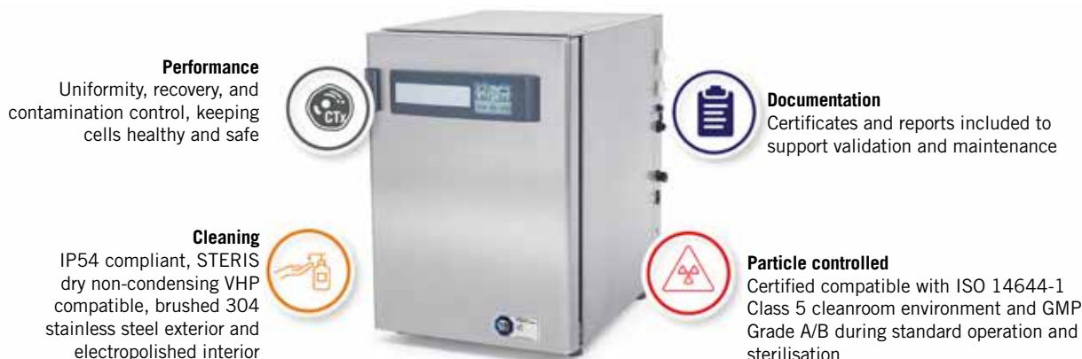
Figure 3: Features of a CO 2 incubator certified for cleanroom use
