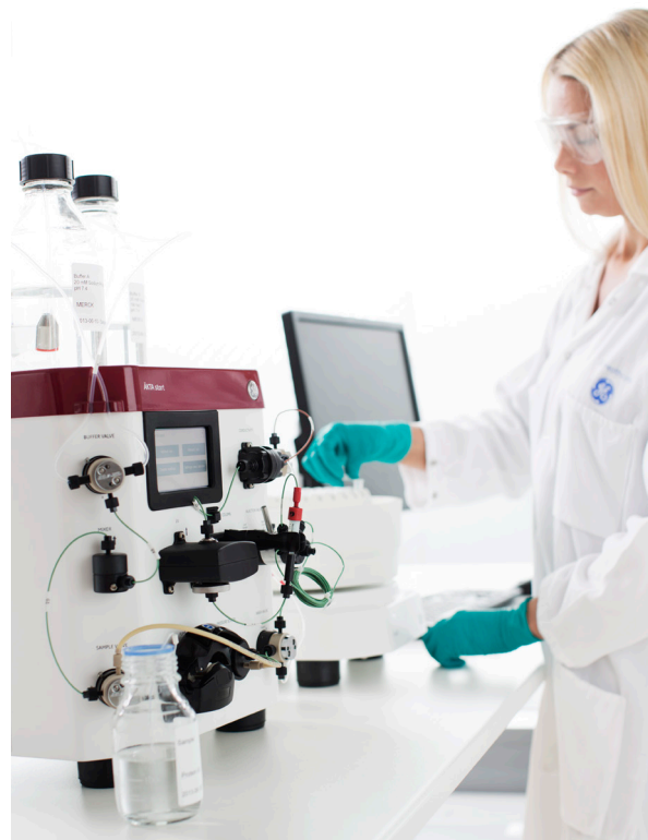
Fig 1. ÄKTA start is an easy-to-use preparative chromatography system designed to facilitate the move into automated protein purification.
